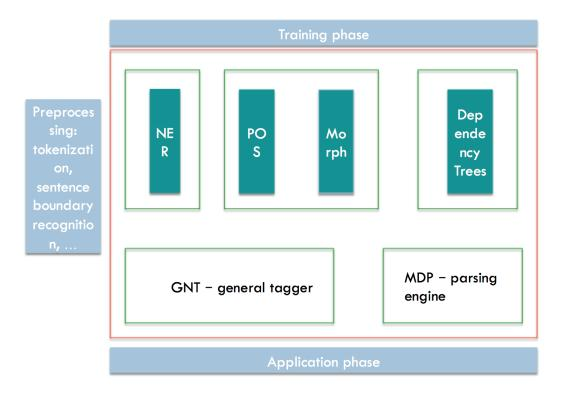
Figure 1: Blueprint of the MunderLine architecture. We distinguish a training phase and an application phase.
